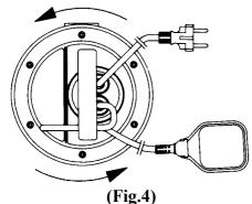
The direction of rotation must be checked each time a new installation is made.
