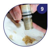
Remove the strainer and cartridge and clean. Check the filter for any remaining debris.
