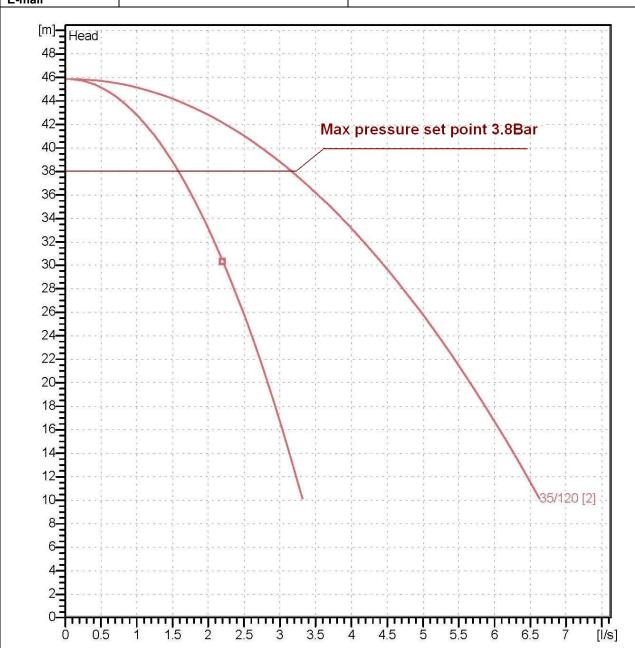
Adjustable working pressure range between 1.0 and 3.8 Bar (10 and 38 Mtrs)
