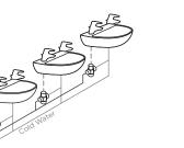
The BOSS thermostatic mixing valves MUST be installed in an accessible position to ensure that maintenance, commissioning and testing of the thermostatic mixing valves can be undertaken easily.
