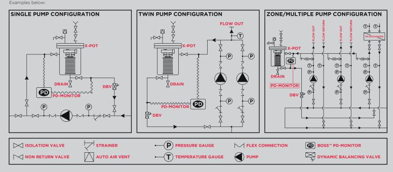
3) The X-POT inlet pipework must be piped from the system pump(s) discharge to X-POT, Entry/Supply Valve (7) and return to pump suction side or a common return line in the system. The maximum pipe run lengths from the system pipework to the X-POT is to be <5m. In the event of multiple zone/pump configurations, a isolation valve and double check valve should be installed on each of the individual pipe runs from the circulating pumps.
